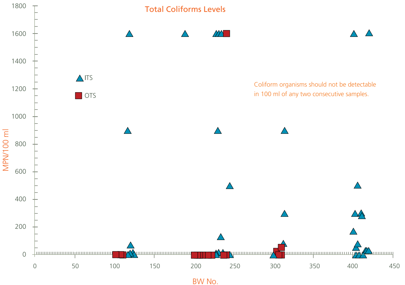
Figure 12: Comparison of total coliform levels of inside town and outside town wells
